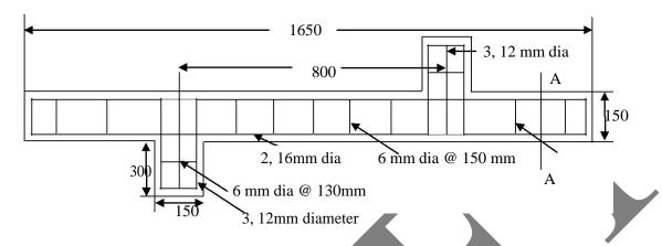
Figure 1: Top view of Torsional Beam
